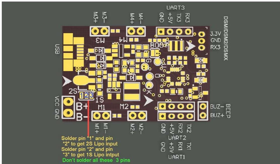
Micro USB socket: Connect to computer to flash firmware and configure the flight controller
