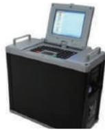
On-line flue gas detector
