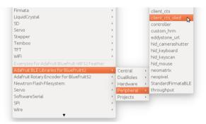
With the sketch loaded, you can build the firmware and then flash it to your device via the Upload button or menu option. Once the sketch is running on the nRF52 Feather you can proceed with the one-time pairing process, described below.
