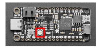
The NeoPixel LED is located between the SWD header and the reset button.
