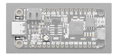
Above the pin labels for A0 and A1 is the status NeoPixel LED. In CircuitPython, the NeoPixel is board.NEOPIXEL and the library for it is here (https://adafru.it/wby) and in the bundle (https://adafru.it/ENC). The NeoPixel is powered by the 3.3V power supply but that hasn't shown to make a big difference in brightness or color. In CircuitPython, the LED is used to indicate the runtime status.
