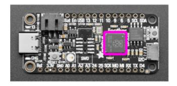
The microcontroller on the Feather RP2040 is located to the right-center of the board, nested between the Adafruit Feather RP2040 label on the silk.
