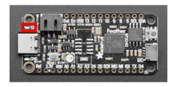
The built-in LED, indicated by the red box in the image, is labeled "13", and located above the USB Type-C connector next to the JST battery connector.
