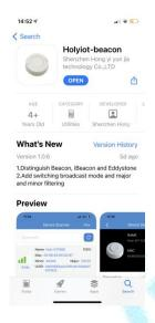
2. Power the module, and turn on Bluetooth, then open the "Holyiot-beacon", you will see detailed beacon advertising information. In the "Beacon" interface, you can see the advertising name, RSSI, MAC, Major, Minor, UUID and remaining battery of the device, and you can filter the signal strength by clicking "Filter", APP supports changing the adversiting type of search, Users can change the search advertising type arbitrarily to scan the corresponding type of advertising equipment.
