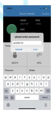
5. After connecting, you can modify the password, Major, Minor, MAC, UUID, broadcast name, transmit power and broadcast interval, and you can also verify the RSSI value at 1 meter. After the adjustment is successful, there will be a "Modify success" prompt, and it will be updated automatically after disconnection.
