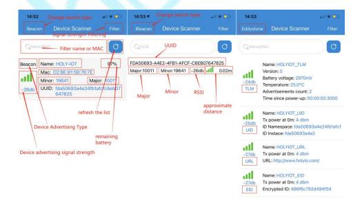
3. In the generic beacon interface, click to select this device, You can see the temperature, air pressure, humidity, whether there is vibration within 20S, button status and power data will be refreshed to the list, provided that the device supports the update of these data.
