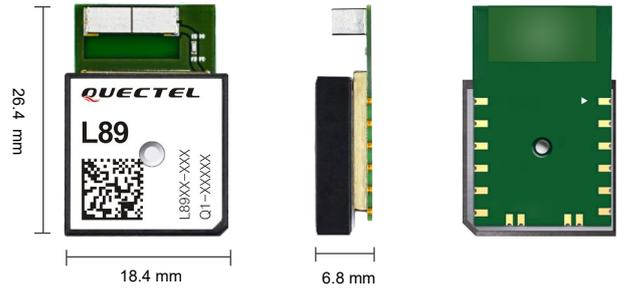
L89 is a high performance IRNSS-enabled GNSS module, capable of acquiring and tracking GPS, IRNSS, GLONASS, BeiDou, Galileo and QZSS signals. With 2 embedded antennas, the module can work at L1 and L5 bands simultaneously.
