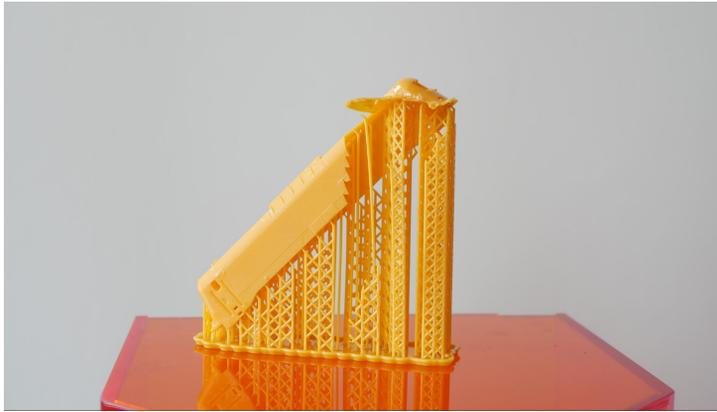
**Solution:** Try printing one of the sample objects to see whether the issue remains. If the sample object was printed without trouble, reset your PrusaSlicer settings. If the sample object has the same sort of trouble, inspect the FEP film in the resin tank - it may be dirty. In very rare scenarios, a faulty UV LED panel can be the cause.
