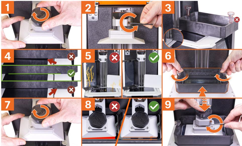
1. Make sure the print platform is clean, slide it onto the platform holder on the cantilever and tighten the black knob.
