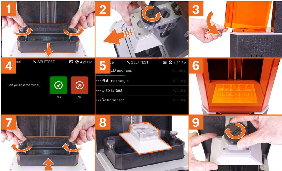
1. Remove the resin tank
