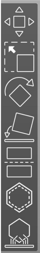
**Move tool (M)** - moves the object in XYZ axes. Click and drag the object to move it in XY axes, use the blue arrow to move it in Z axis (up and down).
