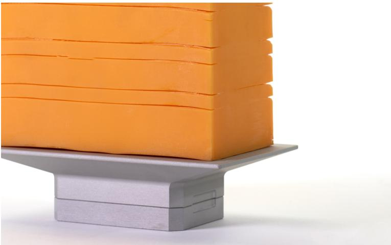
**Solution:** This printing error is caused by the physical properties of resins. Consider hollowing problematic objects, if you encounter layer warping.
