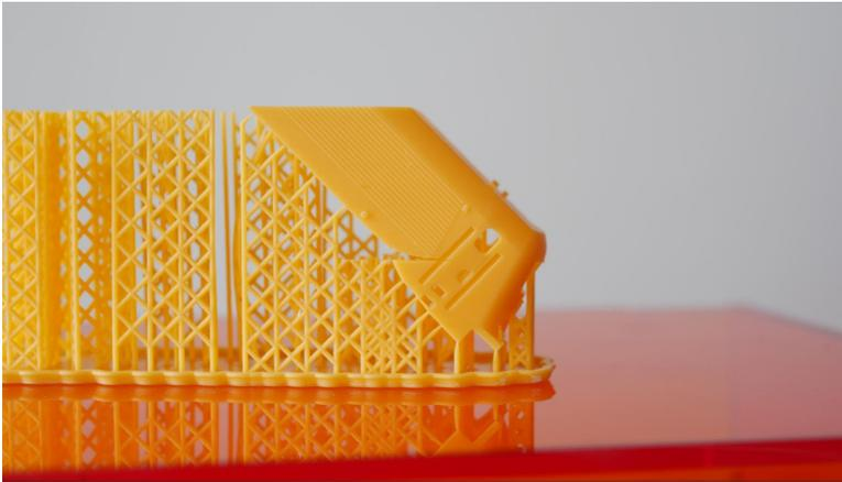
**Solution:** Try printing a sample object and see if the issue persists. If it does, clean the resin tank properly and try again. Continuous issues with separated / missing layers can be caused by a faulty UV LED panel - check whether it works correctly. Otherwise, the cause is most likely a broken object file. Either try re-slicing the model or download a new one.
