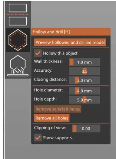
**Adding drainage holes** - Drainage holes can be added by left-clicking on the object when the SLA hollowing gizmo is active. The holes can later be repositioned by dragging them on the mesh. You can remove holes by right-clicking on any of them.
