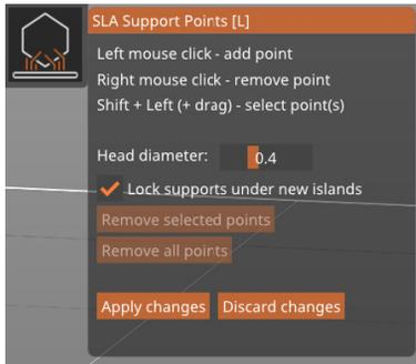
Clicking the Manual editing button opens a new menu and a new set of tools, which enable you to manually add, remove and modify support points on the object. Use Left mouse click to add a support, right mouse click to remove a support, and combine Shift+Left mouse to drag a selection box to select more supports. You can left-click and drag a support point to reposition it.
