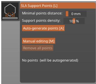
In the picture on the left is the **SLA Support Points** menu, which can be found in the left-side toolbar. If you can't open it, it usually means the model you have imported is too large for the print bed. Move, rotate and scale the object so it fits - the object should be displayed in green colour.
