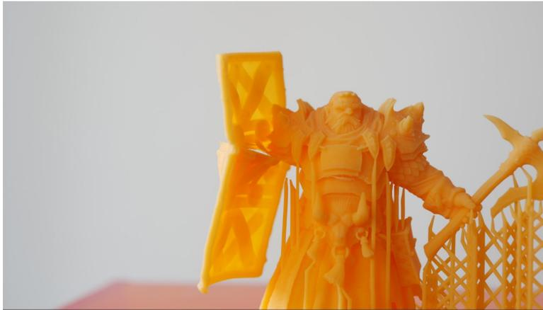
*The warrior's right arm is missing completely and a part of the shield is damaged*
