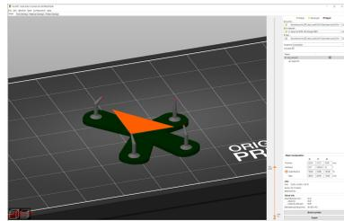
**Part of an object starting mid-air.** PrusaSlicer can recognize these issues almost every time - these errors usually appear if you manually delete an important support point. You can fix it by re-generating the supports or by adding support points manually.
