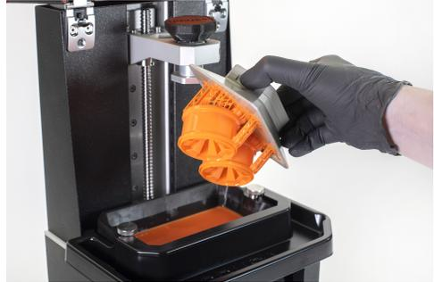
Use the **bundled metal spatula** to remove the print from the print platform. To prevent injuries, **do NOT use your fingernails** to remove the prints since the plastic can easily get under your nails and break off.
