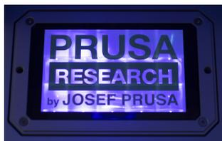
! Use a **soft paper towel** or cloth and an LCD screen cleaning spray to clean the protective glass
