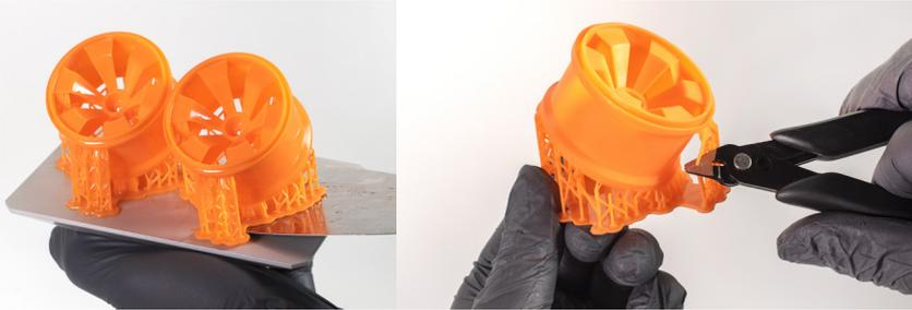
Use a metal spatula to remove the printed object from the printing platform. You can also consider removing the supports at this point.
