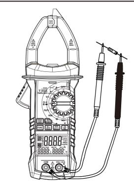
Figure 5 Schematic Diagram for Diode Testing at (Ωον) Gear
