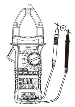
Figure 3: Schematic Diagram for Frequency Measurement at HZ% Gear
