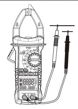
Figure 6 Schematic Diagram for Circuit Continuity Test at ↔ Gear
