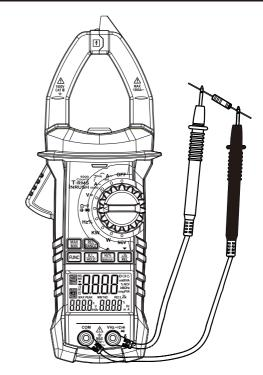
Figure 4 Schematic Diagram for Resistance Measurement at  $\stackrel{\Omega^{(0)}}{H}$  Gear
