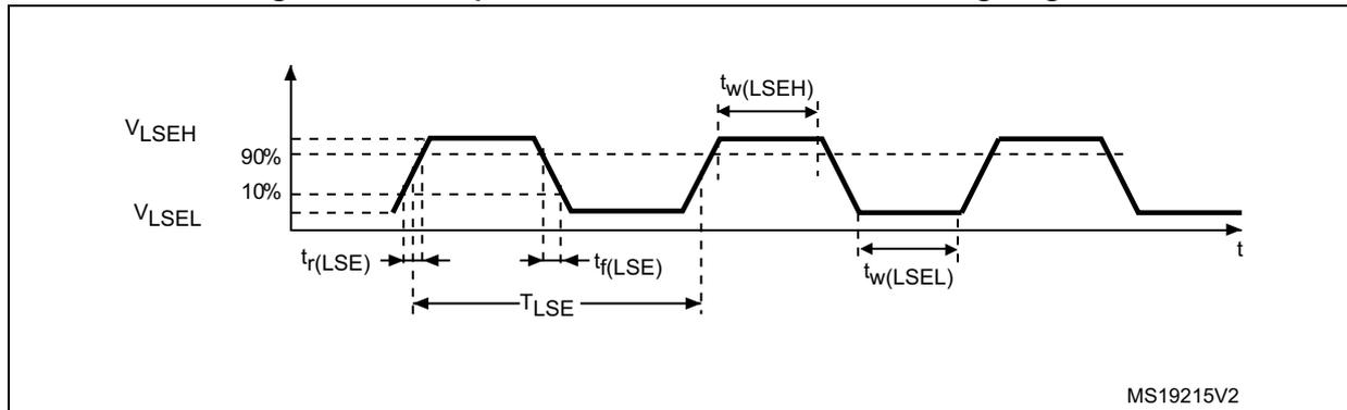
Table 55. Low-speed external user clock characteristics<sup>(1)</sup> – Bypass mode
