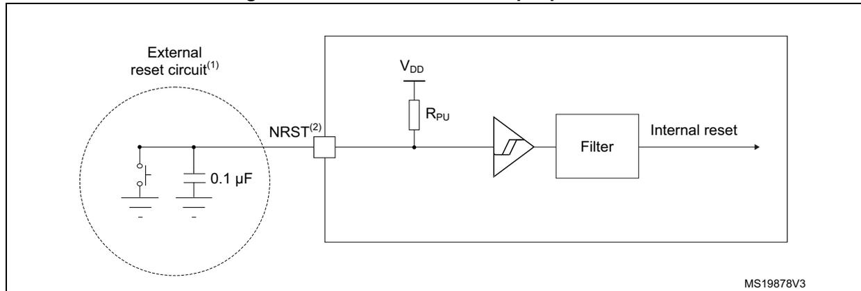
1. The reset network protects the device against parasitic resets.
