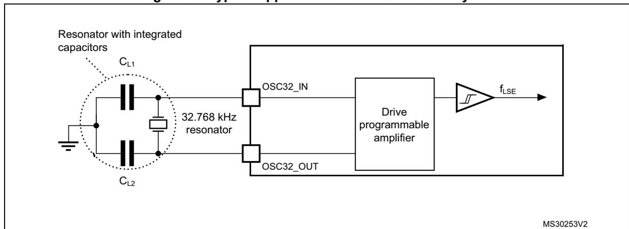
**Note:** No external resistors are required between  $OSC32\_IN$  and  $OSC32\_OUT$ , and it is forbidden to add one.
