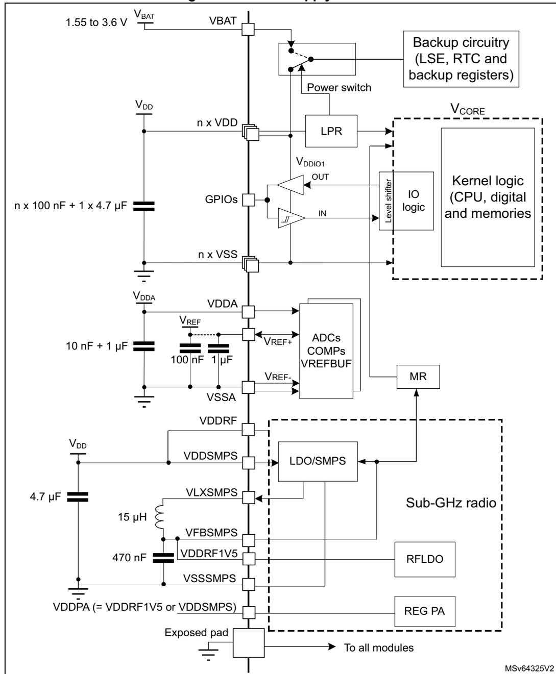
**Caution:** Each power supply pair (such as  $V_{DD}/V_{SS}$  or  $V_{DDA}/V_{SSA}$ ) must be decoupled with filtering ceramic capacitors as shown in the above figure. These capacitors must be placed as close as possible to (or below) the appropriate pins on the underside of the PCB to ensure the good functionality of the device.
