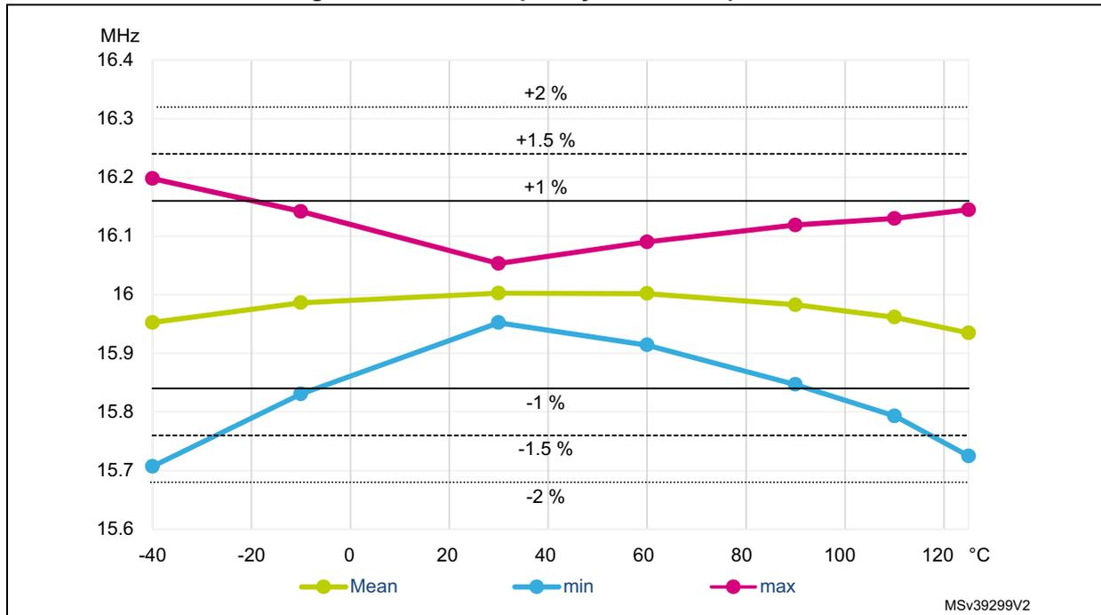
Multi-speed internal (MSI) RC oscillator
