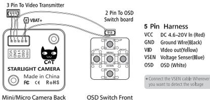
**CAUTION:** If you are using ESC's with active braking, we recommend powering the camera system through a BEC or voltage regulator.
