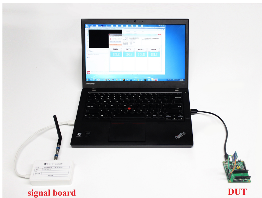
Figure 2-4. Quick Start on Testing Diagram
