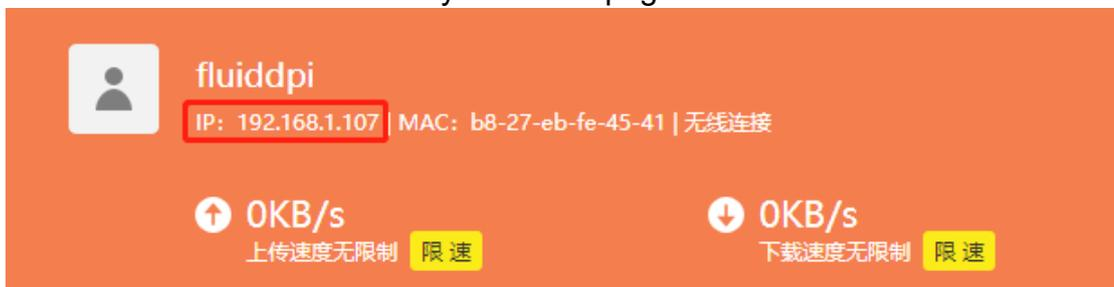
5. Or use the <https://angryip.org/> tool, scan all IP addresses in the current network organize by names, and find the IP named Fluidd, Mainsail (CM4), or BTT-CB1 (CB1), like shown below.
