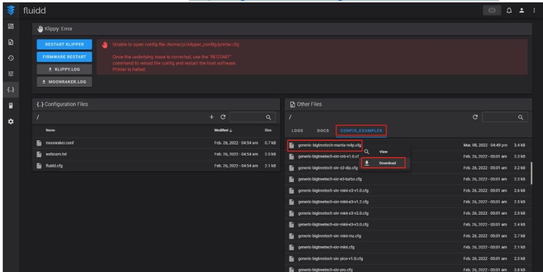
2. Upload your finished config file into Configuration Files, and rename it to "printer.cfg".
