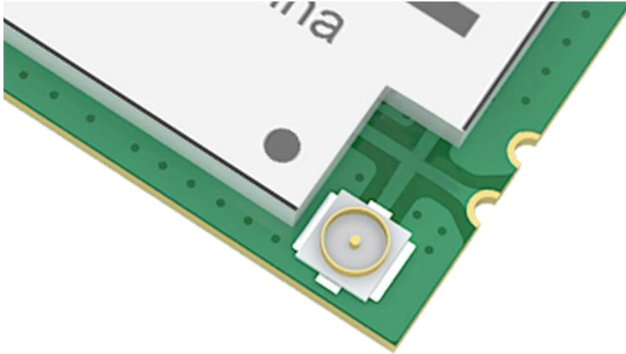
At the same time enable IPEX interface and stamp hole interface, IPEX interface and stamp hole interface can be arbitrarily selected
