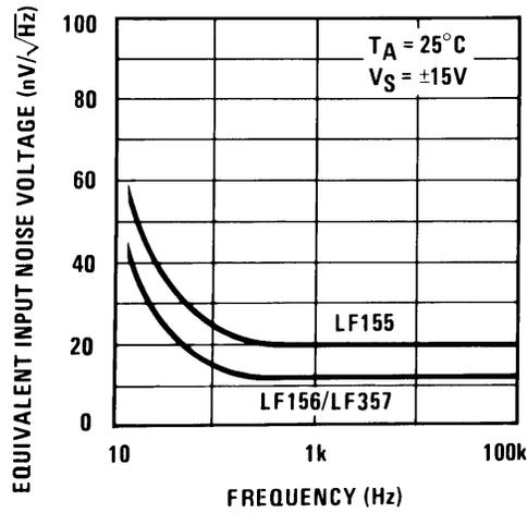
Figure 21. Equivalent Input Noise Voltage (Expanded Scale)
