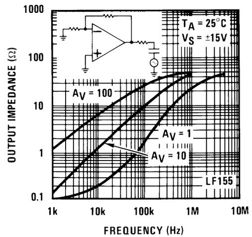
Figure 4. Output Impedance
