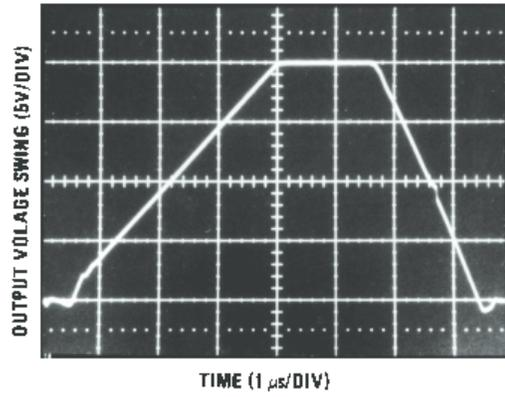
Figure 8. LF155 Large Signal Pulse Response,  $A_V = +1$
