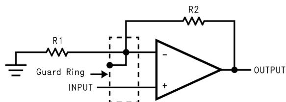
**Figure 36. Noninverting Amplifier**
