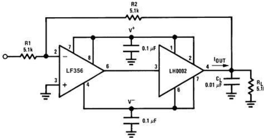
Figure 28. Boosting the LF156 With a Current Amplifier
