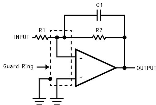
**Figure 35. Inverting Amplifier**
