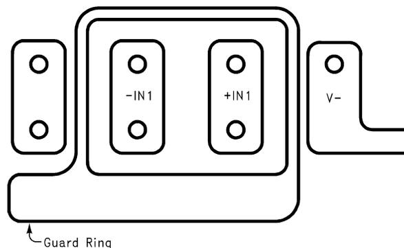
**Figure 39. Examples Of Guard Ring In PCB Layout**
