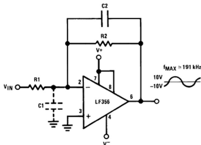
**Figure 27. Wide BW Low Noise, Low Drift Amplifier**
