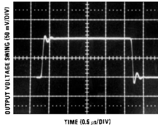
Figure 6. LF155 Small Signal Pulse Response,  $A_V = +1$
