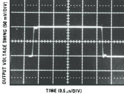
Figure 7. LF156 Small Signal Pulse Response,  $A_V = +1$
