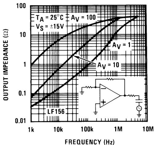
Figure 5. Output Impedance
