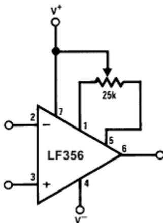
**Figure 33.  $V_{OS}$  Adjustment**
