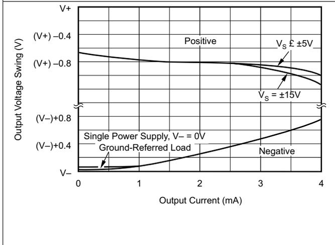
**Figure 15. Output Voltage Swing vs Output Current**
