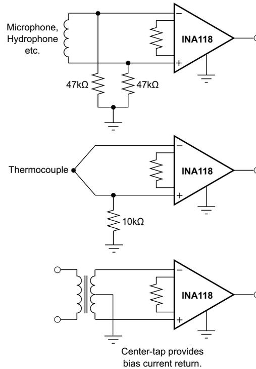
Figure 28. Providing an Input Common-Mode Current Path
