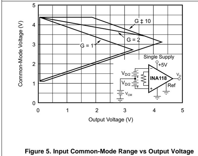
Figure 5. Input Common-Mode Range vs Output Voltage
