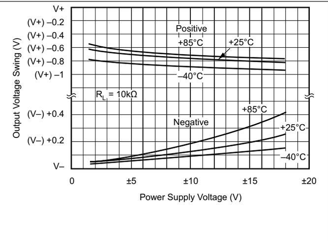
**Figure 16. Output Voltage Swing vs Power Supply Voltage**
