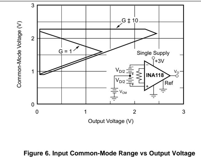
Figure 6. Input Common-Mode Range vs Output Voltage
