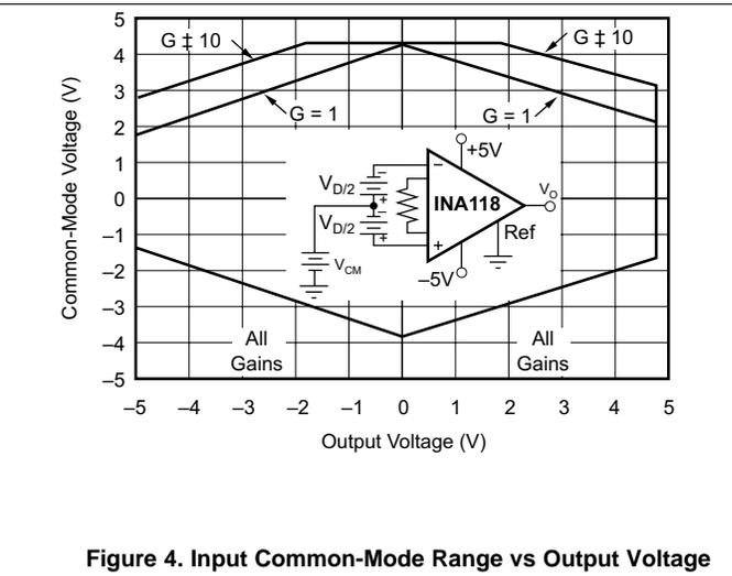
Figure 4. Input Common-Mode Range vs Output Voltage
