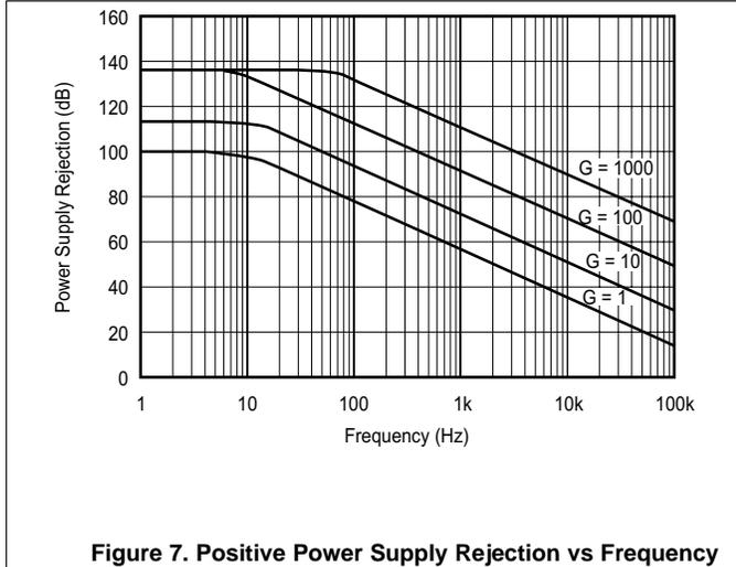
Figure 7. Positive Power Supply Rejection vs Frequency
