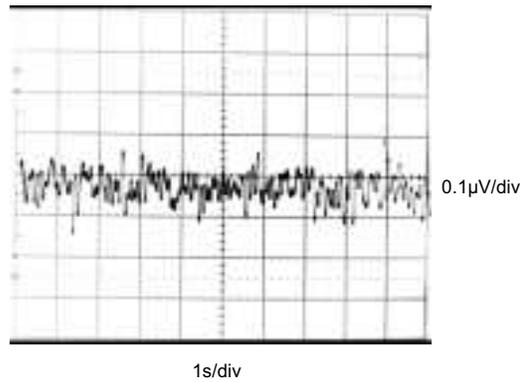
Figure 20. Input-Referred Noise, 0.1 Hz to 10 Hz
