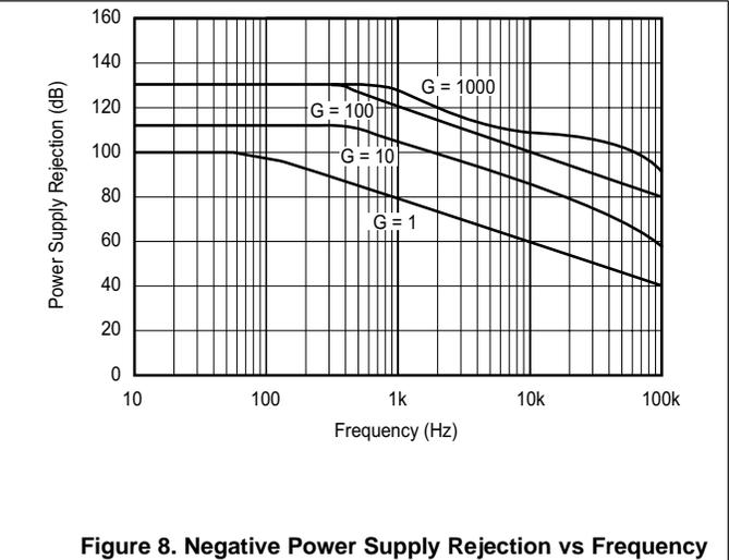
Figure 8. Negative Power Supply Rejection vs Frequency
