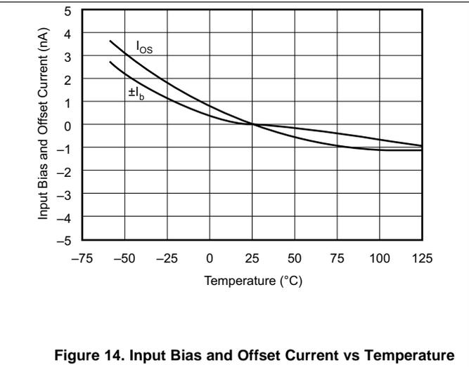
**Figure 14. Input Bias and Offset Current vs Temperature**
