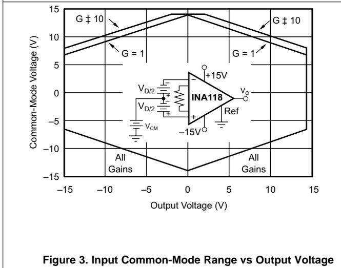
Figure 3. Input Common-Mode Range vs Output Voltage
