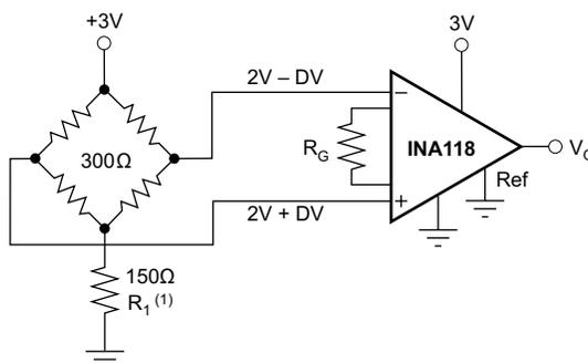
NOTE: (1)  $R_1$  required to create proper common-mode voltage, only for low voltage operation — see text.
