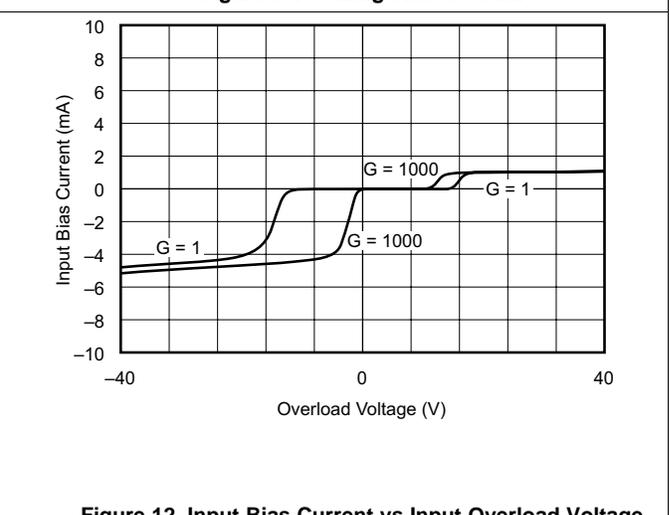
Figure 12. Input Bias Current vs Input Overload Voltage
