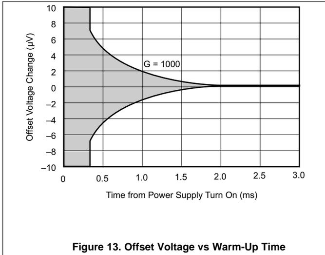
**Figure 13. Offset Voltage vs Warm-Up Time**
