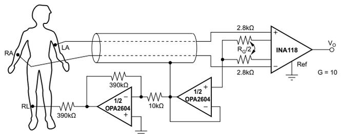
**Figure 34. ECG Amplifier With Right-Leg Drive**
