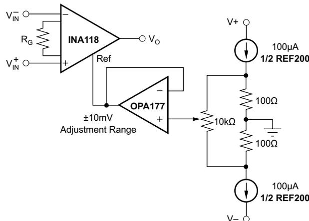
**Figure 27. Optional Trimming of Output Offset Voltage****9.2.2.4 Input Bias Current Return Path**
