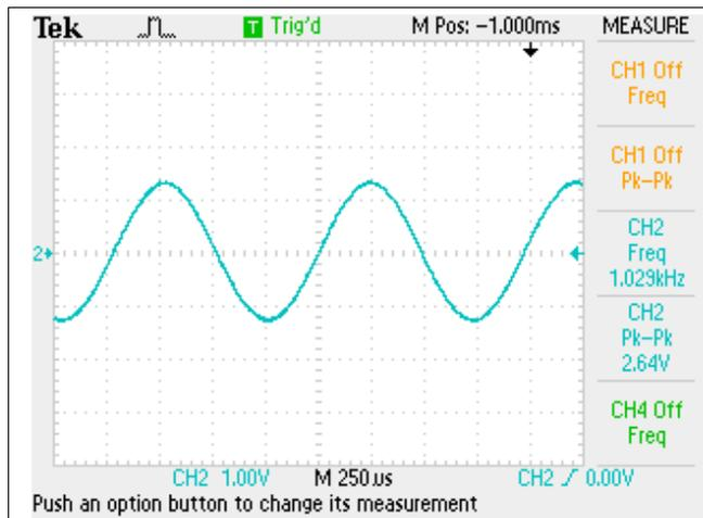
1-kHz differential signal is also present but cannot be seen in this waveform.
