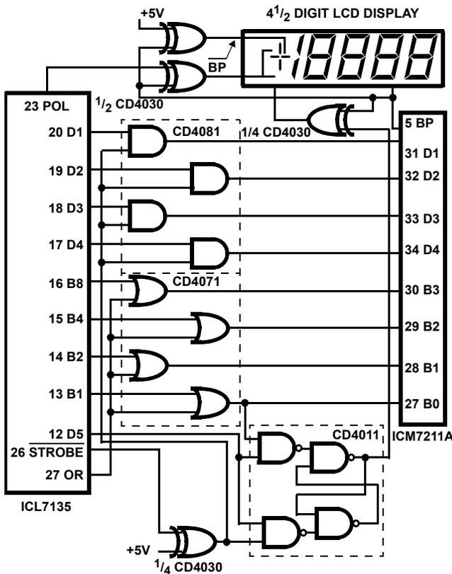
FIGURE 9. LCD DISPLAY WITH DIGIT BLANKING ON OVERRANGE
