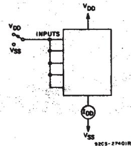
Fig. 9 — Quiescent device current test circuit.
