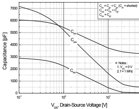
**Figure 5. Capacitance Characteristics**
